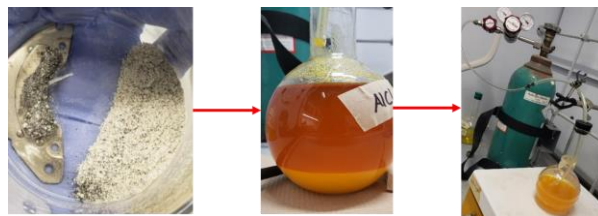
Figure 1. Acid leaching of a lunar highlands simulant. The picture shows the three most important steps of the process. The picture on the left shows the magnetic beneficiation of the simulant. The picture on the center shows the resulting precipitate and supernatant solution after leaching. The picture on the right shows the sparging step to force the precipitation of ACH.
